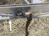
Note: We believe the damage shown was caused by rough water created by boat wakes rather than during a docking procedure
